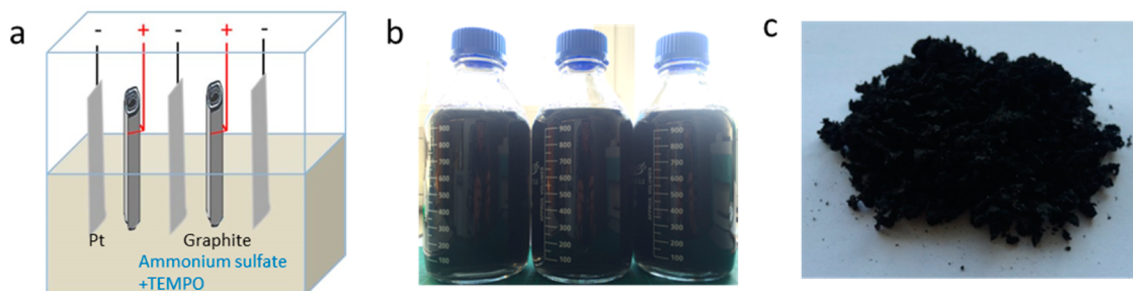
Figure 1. Electrochemical exfoliation of graphite: (a) schematic illustration of an electrochemical cell, (b) stable graphene-DMF dispersions prepared from radical-assisted electrochemical exfoliation, and (c) dried graphene powder ( \sim 15.1 g).
